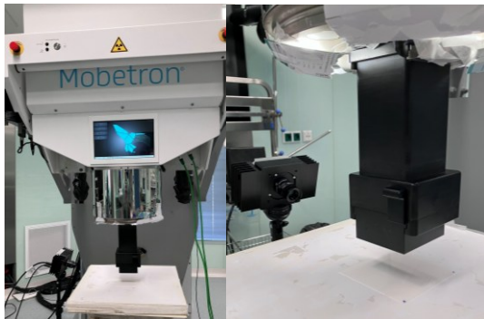
Figure 1. BrightEye dosimetry system setup tested on the IntraOp capable of delivering 6MeV and 9MeV UHDR beams, equipped with two beam current transformers (BCTs) .
